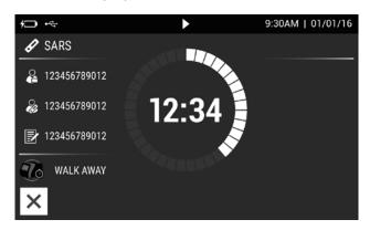
For example: This display shows that the test in WALK AWAY Mode has 12 minutes, 34 seconds remaining. Sofia 2 will read and display the results in 15 minutes.
