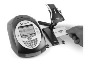
2. Input the Patient ID or Order # using the barcode scanner or manually enter the data using the key pad.
